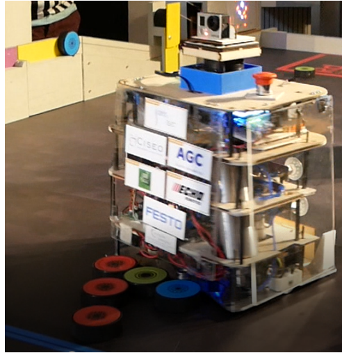
Figure 17: Robot uses the bottom plate to collect atoms
